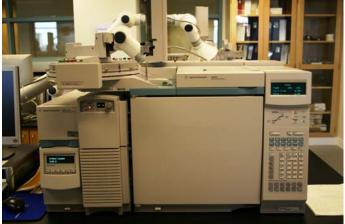
The Agilent Technologies 6890N Network GC System is use by lab technicians to test samples from the study and provide the supporting data for this report.
